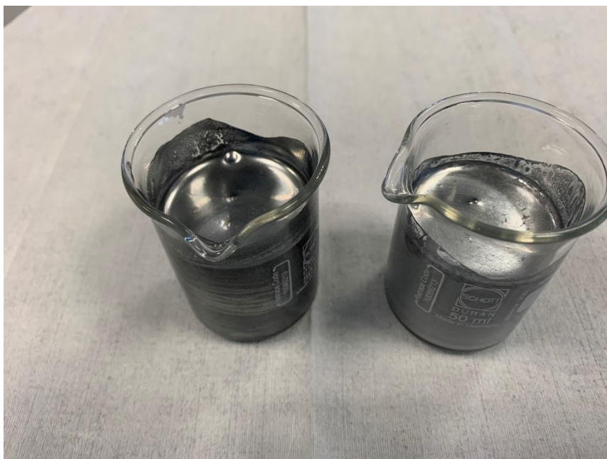
Figure 2: Already diluted Pigment dispersions „Hydroshine“ and „Mirrorshine“. Only 1-2 drops of these are required for analysis.
