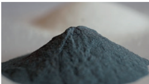
Graphite powder measured with BELPYCNO L, density = 2.223\text{g/cm}^3
