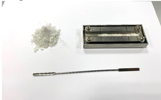
Figure 10: Fine glass powder on the sample holder (approx. 100 mg)
