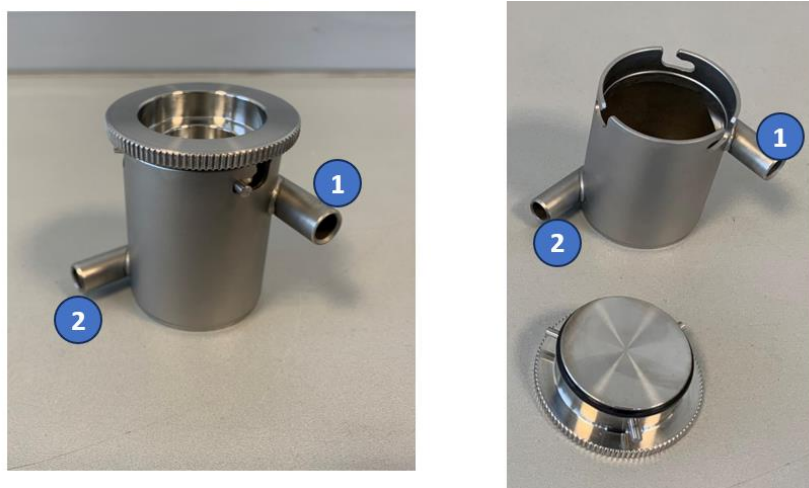
Figure 3: Typhoon accessory. Sample inlet (1), sample outlet (2). Left: closed and locked Right: shutter cover opened
