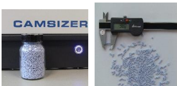
Fig.2: A sample of extruded catalysts. The CAMSIZER 3D image analyzer measures 250 ml in 3 minutes, manual measurement with the caliper analyzes approx. 200 particles per hour.
