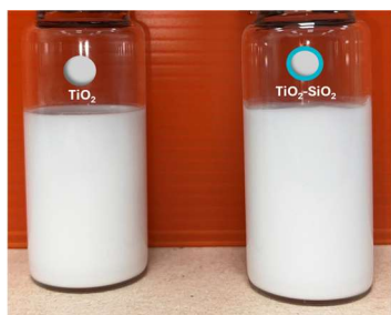
Figure 5: Destabilization not detected by naked eye
