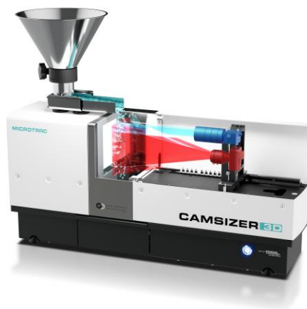
Figure 1: Measuring principle of CAMSIZER S1 and CAMSIZER 3D. The sample is fed into a funnel and transported to the measuring zone via a vibrating chute. The particles are detected and evaluated as shadow projections in free fall. This design is suitable for free-flowing bulk solids. The two CAMSIZER models differ in their measuring range and camera equipment.
