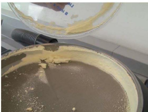
Fig.7: Powdered cream on a 63 µm sieve after one minute air jet sieving
