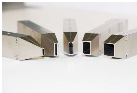
Fig. 2: CAMSIZER X2 measurement principle (left). Particles are dispersed in an air flow and more than 300 images / second of the moving particles are acquired by two cameras. The default nozzle has 4mm aperture (right image, middle nozzle). Large nozzles are available for bigger particles.
