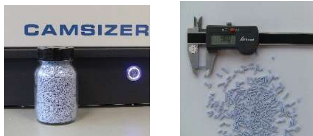
Fig. 5: Extruded catalyst sample. Advantage CAMSIZER P4: 250 ml analyzed in 3 minutes, Caliper: 200 pieces in 1 hour
