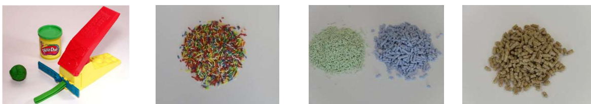
Fig. 1: The process of extrusion (left) creates elongated particles: e. g. sugar sprinkles, catalyst carriers or animal feed (from left to right).
