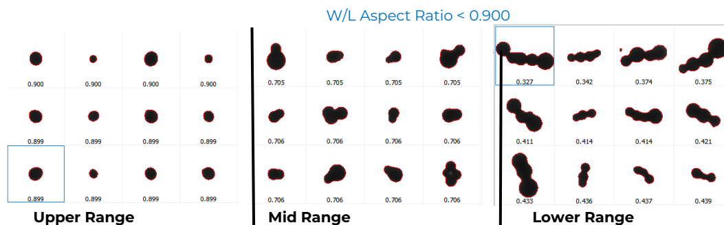
Figure 14. Selected images in W/L range less than 0.900. As W/L decreases, images show increasingly fused individual powder particles. QC departments can use images as guides for setting their specifications on shapes.
