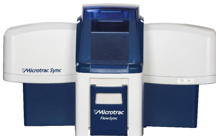
Figure 1. Synchronous Size and Shape Analyzer: Each measuring unit measures and reports all results simultaneously on the same sample. The instrument pictured measures one sample using both the Laser Diffraction and Dynamic Image Analysis technologies.
